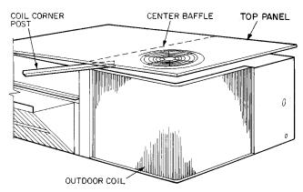
Fig. 22 — Propping Up Top Panel
